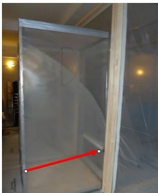
Photo 1 : Photograph of a "cube" attached to an enclosure. The cube is a single stage airlock measuring 1m x 1m x 2m fitted with door openings and flaps identical to one stage of a 3-stage airlock. Photo shows the door flap with full scale deflection.
