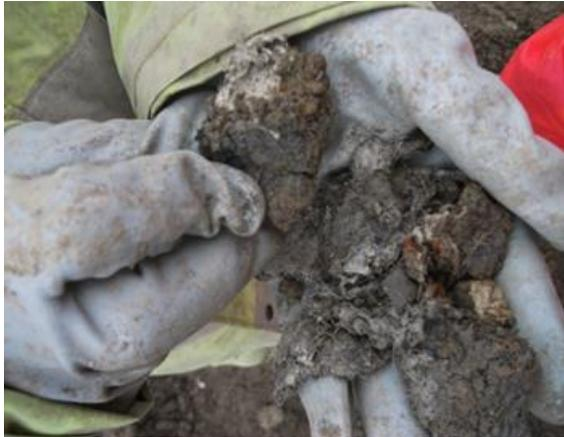
Photo 1. Degraded asbestos material not identifiable as its original product.
